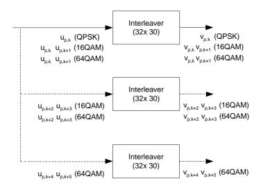
Figure 18: Interleaver structure for HS-DSCH
